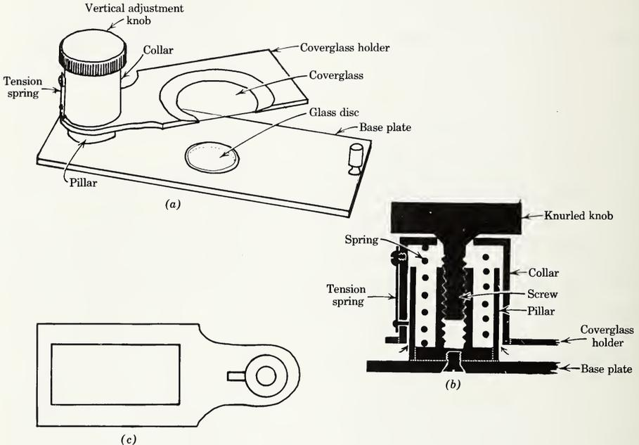
**Fig. 46.1.** Compressor of the type formerly made by Watson & Sons. (a) General view. In use the adjustment knob would be to the right for a right-handed person. (b) Vertical section of adjustment mechanism. (c) Suggested improved form of coverglass holder.
