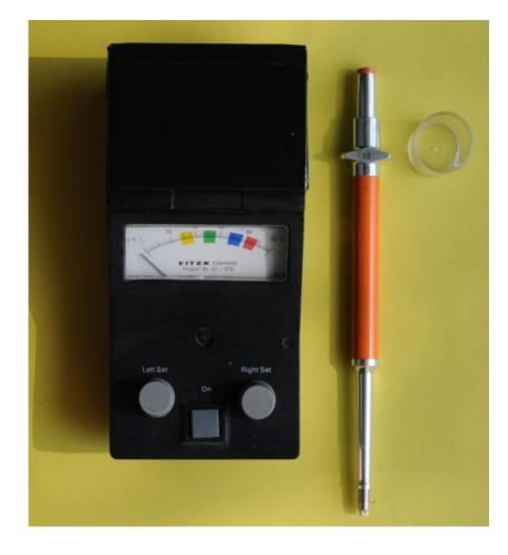
Densitometer allowing the measurement and the adjustment of spores suspensions, in order to standardize the quantity in the sampling probe.
